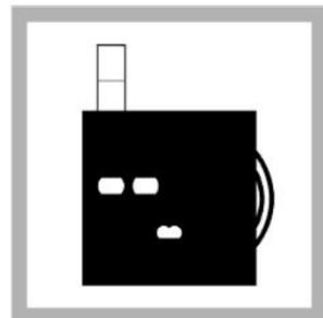
Put one tube into the left opening of the color comparator box. Ensure your materials are oriented like the diagram above.
