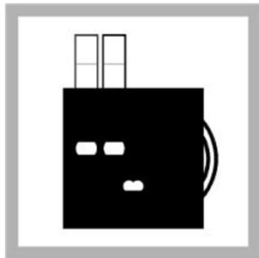
Put the second tube into the color comparator box.
