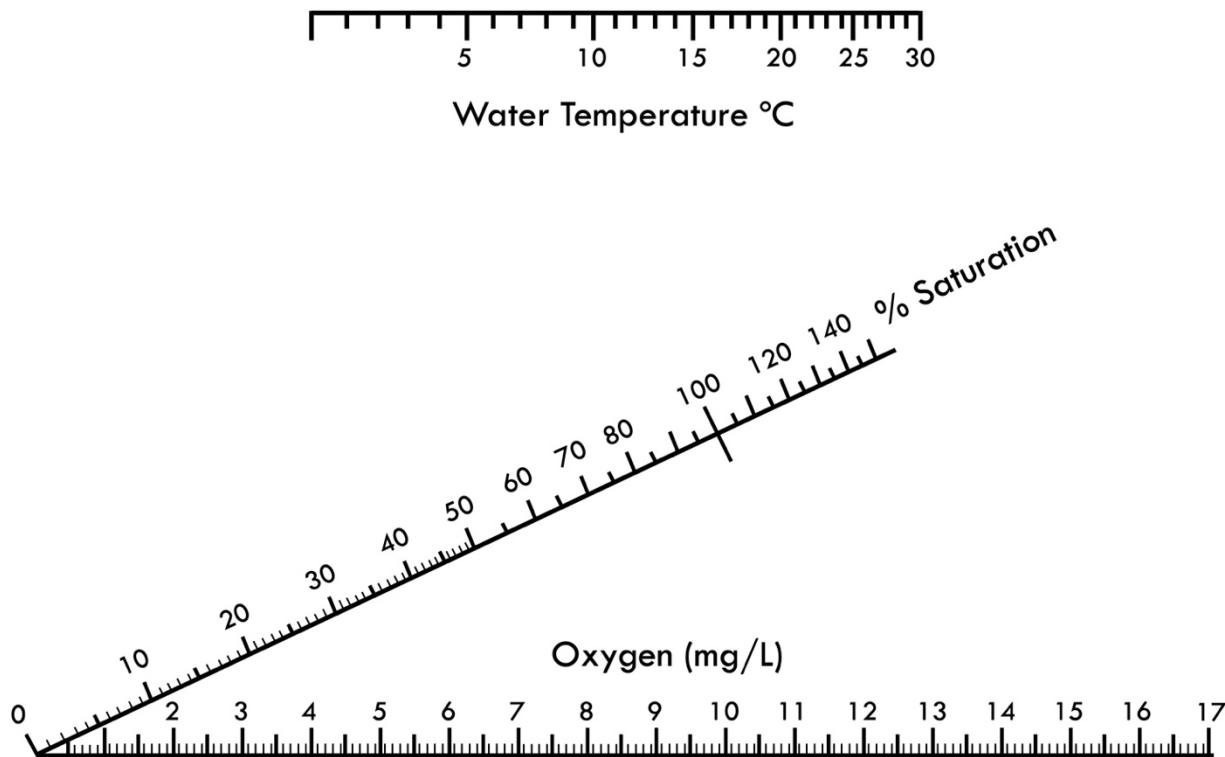
To use the nomogram, use a ruler or straight object to draw a line from your temperature value (at the top) to your dissolved oxygen value (at the bottom). The point at which that line crosses the saturation line is your percent saturation. Example:
