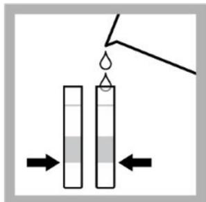
Fill two tubes to the 5 mL line (bottom of shaded area) with sample. See diagram above.
