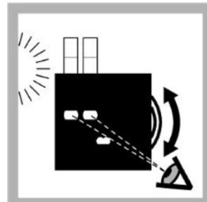
Hold the color comparator box in front of a light source. Turn the color disc to find the color match.
