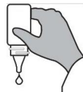
Hold dropper bottles vertically upside-down, and not at an angle when dispensing reagent. Squeeze the bottle gently to dispense the reagent one drop at a time.
