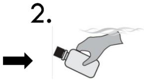
Tightly cap the bottle, then submerge it to the desired depth.
