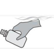
While bottle is underwater, remove the cap and allow the bottle to fill.
