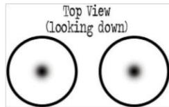
Check the turbidity again by looking down through the tubes at the black dots. Repeat this process and count the number of times you complete Step 6 until both dots appear the same.
