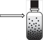
Allow the precipitate to settle below the shoulder of the bottle.
